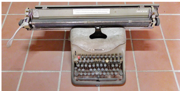
Fig. 2 Typewriter for Typing Palm-Leaf Manuscripts (photo by Silpsupa Jaengawang, Vat Suvanna Khili, Luang Prabang, August 24, 2022)
